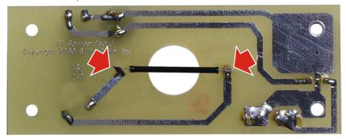
2. Carefully slip the wires of the one inch bulb from the clips
