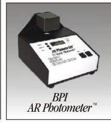
One minute after calibration the unit will shut itself off (display dashes); push the Calibrate button to reset. The display will show the UV, AR quality and visible readings until the READ or CAL buttons are pressed or until the maximum calibration period elapses.
